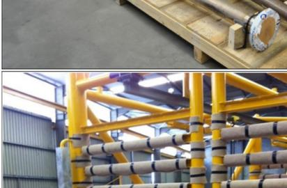
Changing temperatures during operation of the Cooling Skid meant that the thermal efficiency of the paint controlled by the limited thickness and anti-fouling properties became key drivers to the success of this work.
